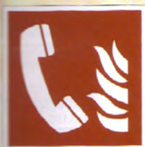
Brandmeldertelefon (ASR A1.3)
